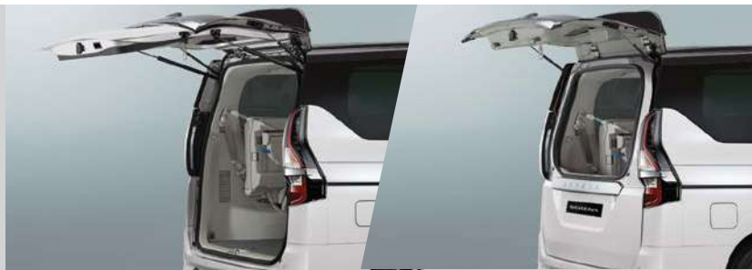
DUAL BACK DOOR making it easier to access the boot in tight spaces.
