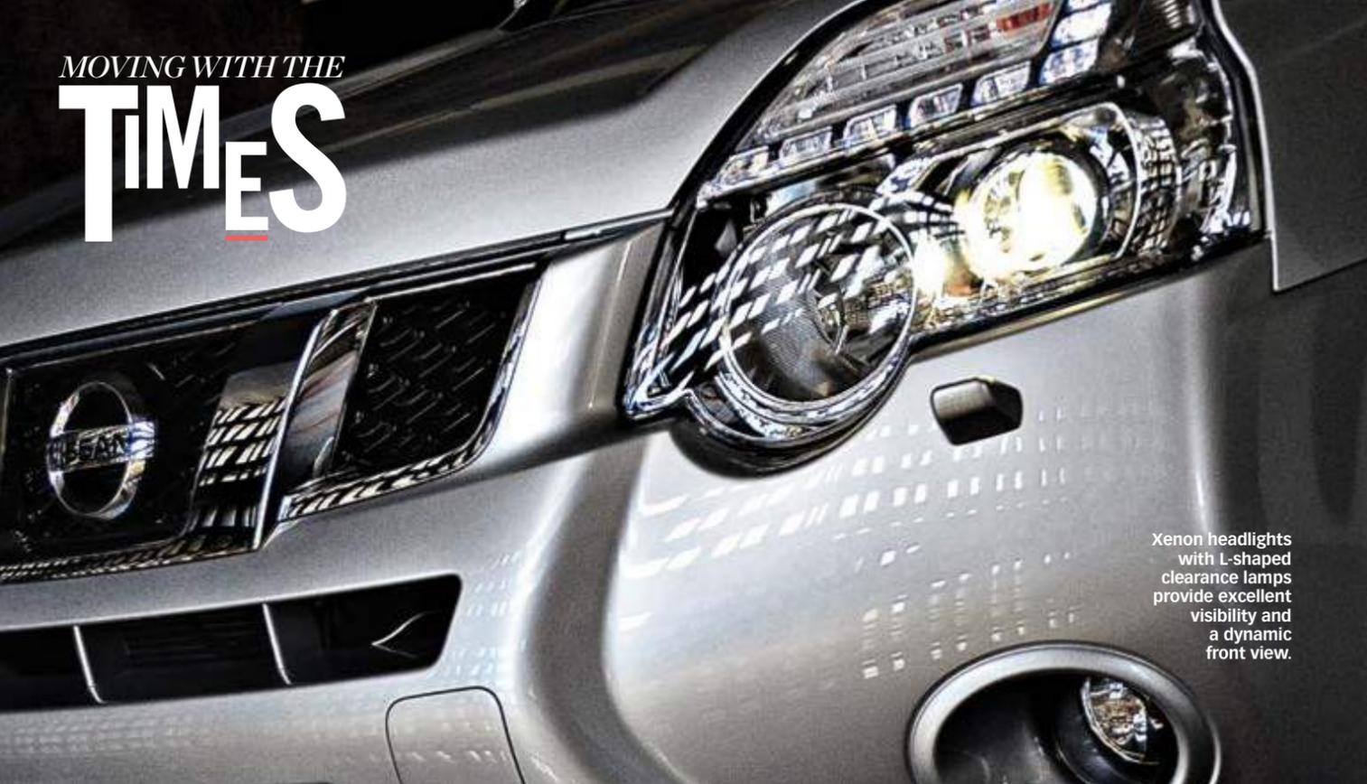
Xenon headlights with L-shaped clearance lamps provide excellent visibility and a dynamic front view.
