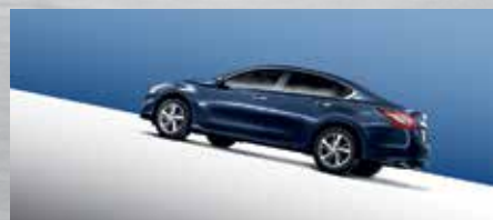
Hill Start Assist (HSA) prevents backward roll on a slope
