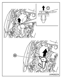
Remove the window washer fluid reservoir if necessary.
