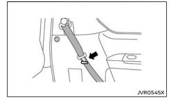
Seat belt can be hooked on the belt hook.
