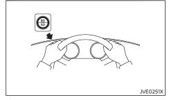
Remove the speed restriction sticker from the tire sealant bottle, then put it in a location where the driver can see it while driving.
