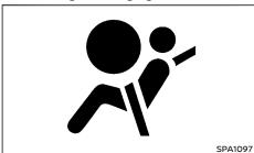
The SRS air bag warning light, displaying \* in the meter, monitors the circuits for the air bag systems, pre-tensioner seat belt systems and all related wiring.
