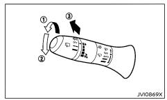
The rear window wiper and washer operates when the ignition switch is in the "ON" position.
