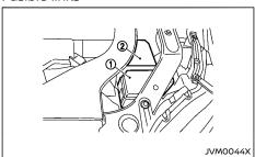
If any electrical equipment does not operate and the fuses are in good condition, check the fusible links in the holders ①, ② and battery terminals. If any of these fusible links are melted, replace only with genuine NISSAN parts.
