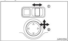
The outside rearview mirror remote control operates when the power switch is in the "ACC" or "ON" position.
