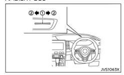
The ambient ECO (1) is displayed according to the accelerator pedal operation, while driving the vehicle in ECO mode.
