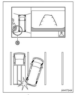
At the position (B) in the bird's-eye view, there seems to be a small distance between the vehicle and the object. However, the actual distance is shorter than the one displayed in the view. The vehicle may hit the object when backing up to the position.
