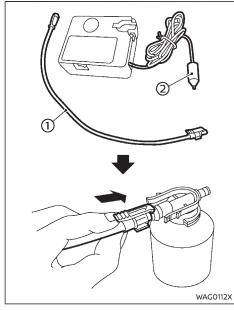
Take the hose ① and the power plug ② out of the air compressor. Connect the hose outlet to the tire sealant bottle securely.
