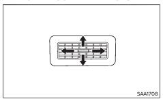
Adjust the air flow direction of the ventilators by moving the center knob (up/down, left/right) until the desired position is achieved.
