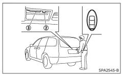
When you carry the Intelligent Key with you, you can lock or unlock all doors by pushing the door handle request switch ① or back door request switch ② within the range of operation.
