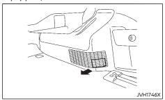
The foot ventilator for the rear air conditioning system is located at the lower left side of the third row seat as shown. (See "Rear air conditioning system" (P.4-18).)
