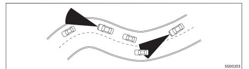
When driving on some roads, such as winding, hilly, curved, narrow roads, or roads which are under construction, the sensor may detect vehicles in a different lane, or may temporarily not detect a vehicle traveling ahead. This may cause the system to work inappropriately.
