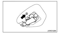
When folding down the third row seat, the center seat belt can be retracted into a stowed position.
