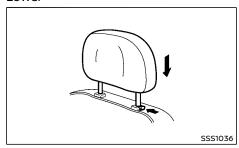
To lower, push and hold the lock knob and push the head restraint down.
