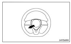
The horn switch operates regardless of the ignition switch position except when the battery is discharged.
