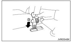
Always be sure the third row center seat belt connector tongue and connector buckle are attached. Disconnect only when folding down the third row seat.
