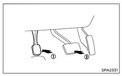
To apply the parking brake, firmly depress the parking brake pedal ①.
