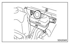
Check the fluid level in the reservoir. If the fluid is below the MIN line ①, the brake warning light will illuminate. Add fluid up to the MAX line ②. (See "Recommended fluids/lubricants and capacities" (P.9-2) for recommended types of fluid.)
