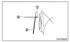
The front-side view is the view from near the front tire on the left side of the vehicle and is displayed on the left side of the screen. The view is useful when the driver needs to park the vehicle on the side of a street.
