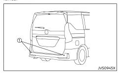
The BSW system uses radar sensors ① installed near the rear bumper to detect other vehicles in an adjacent lane.
