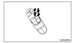
The automatic function is available for the switch that has an  $\boxed{\mathbf{A}}$  mark on its surface.
