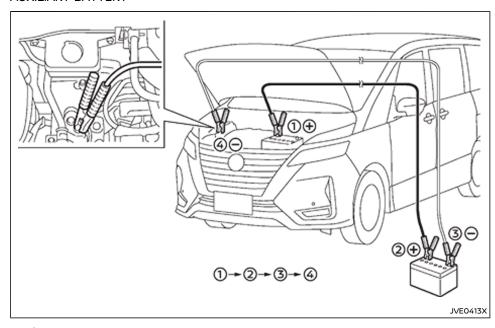
If the booster battery is in another vehicle, position the two vehicles to bring the batteries into close proximity to each other.
