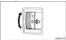
The headlight aiming control operates when the ignition switch is in the "ON" position and the headlight is on to allow the headlight axis to be adjusted according to the driving conditions.
