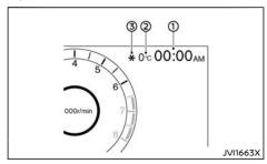
The clock 1 and outside air temperature 2 are displayed on the upper side of the vehicle information display.
