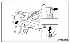
If the battery is discharged, the shift lever may not be moved from the "P" (Park) position even with the foot brake pedal depressed.
