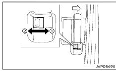
To lock the sliding door without a key, push the lock knob to the lock position ①, and then close the door.
