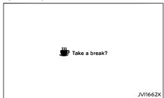
If the system detects that driver attention is decreasing, the message "Take a break?" appears in the vehicle information display and a buzzer sounds when the vehicle is driven at speeds above 60 km/h (37 MPH).
