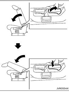
Pull up the adjusting lever to fold the seatback.
