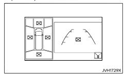
When the "\sum " icon is displayed on the screen, the camera image may be receiving temporary electronic disturbances from surrounding devices. This will not hinder normal driving operation but the system should be inspected by a NISSAN dealer if it occurs frequently.
