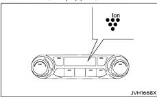
This unit generates highly concentrated Plasmacluster ions into the air blown from the ventilators and reduces odor absorbed into the interior trim.
