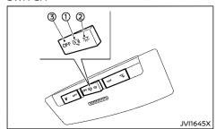
The map/room lights control switch has three positions: DOOR ①, ON ② and OFF ③.
