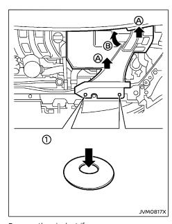
Remove the air duct if necessary.
