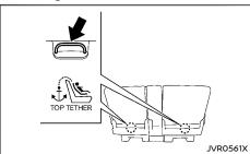
Your vehicle is designed to accommodate a child restraint system on the second row seat. When installing a child restraint system, remove the head restraint. Carefully read and follow the instructions in this manual and those supplied with the child restraint system.
