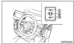
power door main switch (for models with Handsfree slide door function)
