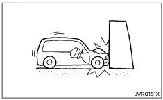
The supplemental front-impact air bag system will deploy in the event of an impact which exceeds a 25 km/h frontal collision with a solid wall that does not move or deform.
