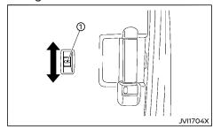
The sliding door's window switch ① can control the corresponding window.
