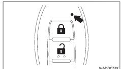
The light (5) blinks only when you push any button on the Intelligent Key. The light illumination only signifies that the Intelligent Key has transmitted a signal. You may look and/or listen to verify that the vehicle has performed the intended operation. If the light (§) does not blink, the Intelligent Key battery may be too weak to communicate to the vehicle. If this occurs, the battery may need to be replaced.
