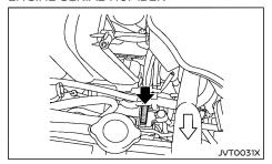
The engine serial number is stamped on the engine as shown.
