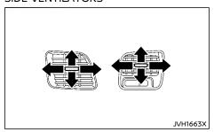
Adjust the air flow direction of the ventilators by moving the center knob (up/down, left/right) until the preferred position is achieved.
