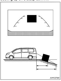
When backing up the vehicle down a hill, the distance guide lines and the vehicle width guide lines are shown farther than the actual distance. Note that any object on the hill is closer than it appears on the monitor.
