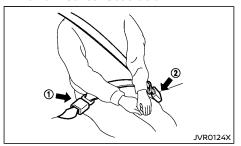
The third row center seat belt has a connector tongue ① and a seat belt tongue ②. Both the connector tongue and the seat belt tongue must be securely latched for proper seat belt operation.
