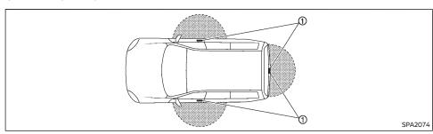
The Intelligent Key functions can only be used when the Intelligent Key is within the specified operating range from the request switch ①.
