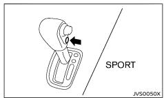
To select the SPORT mode, push the SPORT mode switch with the shift lever in the "D" (Drive) position. The SPORT mode indicator light sporr in the meter panel illuminates. To turn off the SPORT mode, push the SPORT mode switch again. The SPORT mode indicator light will turn off. When the shift lever is shifted to any position other than "D", the SPORT mode will be automatically turned off.
