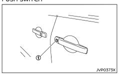
When the sliding door is fully closed/opened, the sliding door will fully open/close automatically by pushing the one-push switch ①.
