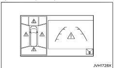
When the " \_\_\_\_\_ " icon is displayed on the screen, there are abnormal conditions in the Around View Monitor. This will not hinder normal driving operation but the system should be inspected by a NISSAN dealer.
