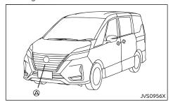
The Intelligent Emergency Braking system uses a radar sensor (a) located on the front of the vehicle to measure the distance to the vehicle ahead in the same lane.
