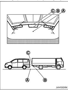
The position © is shown farther than the position ® in the display. However, the position © is actually at the same distance as the position ⓐ. The vehicle may hit the object when backing up to the position ⓐ if the object projects over the actual backing up course.
