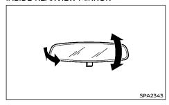
While holding the inside rearview mirror, adjust the mirror angles until the desired position is achieved.
