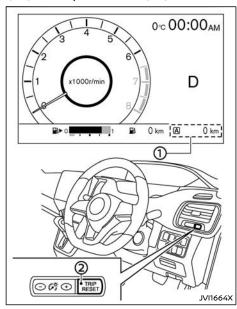
The odometer/twin trip odometer is displayed when the ignition switch is in the "ON" position or placed from the "ON" position to the "OFF" position.
