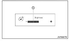
The instrument brightness control switch can be operated when the ignition switch is in the "ON" position.
