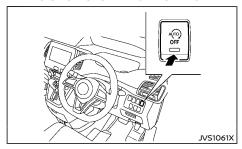
Use the Idling Stop System OFF switch when you would like to stop operation of the Idling Stop System.
