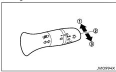
To turn on the high beam, push the lever towards the front position ①.
