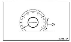
The tachometer, displayed in the vehicle information display, indicates the engine speed in revolutions per minute (rpm). Do not rev the engine into the red zone 1.
