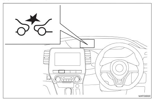
When the radar sensor picks up interference from another radar source, making it impossible to detect a vehicle ahead, the Intelligent Forward Collision Warning system is automatically turned off. The Intelligent Emergency Braking system warning light (orange) will illuminate.
