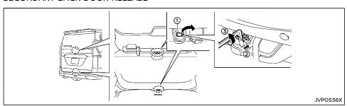
The secondary back door release mechanism allows the back door to be opened in the event of a discharged battery, etc.
