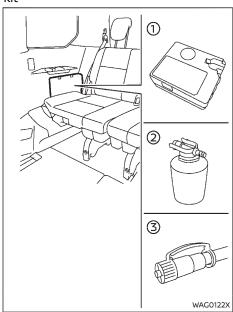
Take out the emergency tire puncture repair kit located on right side of the third row seat. The
