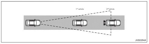
The Intelligent Forward Collision Warning system operates at speeds above approximately 5 km/h (3 MPH).
