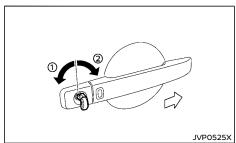
To lock the door, insert the key into the door key cylinder located on the driver's side door, and turn the key toward the rear of the vehicle ①. All doors will lock.
