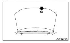
The air conditioner specification label is affixed to the underside of the hood as shown.
