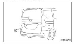
The two radar sensors ① for the BSW system are located near the rear bumper. Always keep the area near the radar sensors clean.
