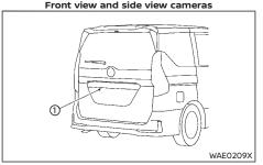
Rear view camera To display the multiple views, the Intelligent
