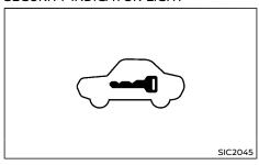
The security indicator light is located in the meter panel. It indicates the status of NATS.
