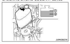
Check the coolant level in the reservoir tank when the engine is cold. If the coolant level is below the MIN level ②, add coolant up to the MAX level ①. If the reservoir tank is empty, check the coolant level in the radiator **when** the engine is cold. If there is insufficient coolant in the radiator, fill the radiator with
