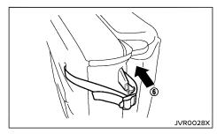
When returning the seat, store the strap (a) and unfold the seat in the reverse order of folding.
