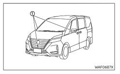
The Intelligent Forward Collision Warning system uses a radar sensor (a) located on the front of the vehicle to measure the distance to the vehicle ahead in the same lane.
