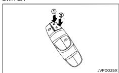
Operating the power door lock switch will lock or unlock all the doors.
