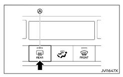
The defogger switch operates when the ignition switch is in the "ON" position.
