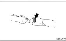
The center seat belt buckle is identified by the CENTER mark. The center seat belt tongue can be fastened only into the center seat belt buckle.
