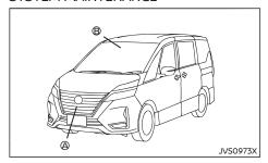
The radar sensor (a) is located on the front of the vehicle. The camera (b) is located on the upper side of the windshield.
