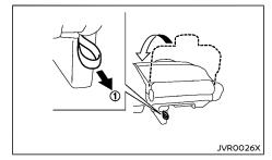
Pull the strap ① to unlatch the seat leg. (The seatback will be folded at the same time.)
