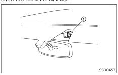
The lane camera unit ① for the LDW system is located above the inside mirror.
