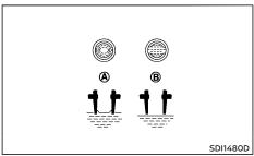
Check the fluid level in each cell. The battery fluid level should be between the UPPER LEVEL ① and LOWER LEVEL ② lines.
