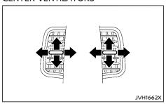
Adjust the air flow direction of the ventilators by moving the center knob (up/down, left/right) until the preferred position is achieved.
