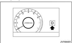
The Continuously Variable Transmission (CVT) position indicator indicates the shift lever position when the ignition switch is in the "ON" position.
