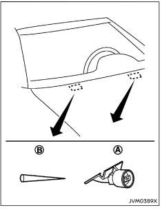
Be careful not to clog the washer nozzle (a). This may cause improper windshield washer operation. If the nozzle is clogged, remove any objects with a needle or small pin (a). Be careful not to damage the nozzle.
