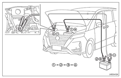
If the booster battery is in another vehicle, position the two vehicles to bring the batteries into close proximity to each other.
