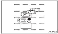
Illustration 5 - Entering from the side Illustration 5: The side indicator light illuminates if a vehicle enters the detection zone from either side.
