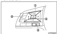
The vehicle information display can be changed using the switches OK 1, 2, 3, and 4 4 @ located on the steering wheel.
