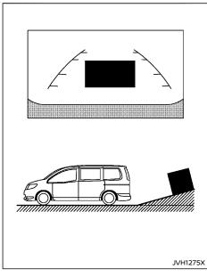
When backing up the vehicle up a hill, the distance guide lines and the vehicle width guide lines are shown closer than the actual distance. Note that any object on the hill is farther than it appears on the monitor.
