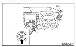
When the ignition switch is pushed without depressing the brake pedal, the ignition switch will illuminate.
