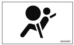
The supplemental air bag warning light, displaying in the instrument panel, monitors the circuits for the air bag systems, pre-tensioner seat belt system (if equipped) and all related wiring.
