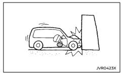
The supplemental front-impact air bag and driver's knee air bag (if equipped) systems will deploy in the event of an impact which exceeds a 25 km/h (16 MPH) frontal collision with a solid wall that does not move or deform.
